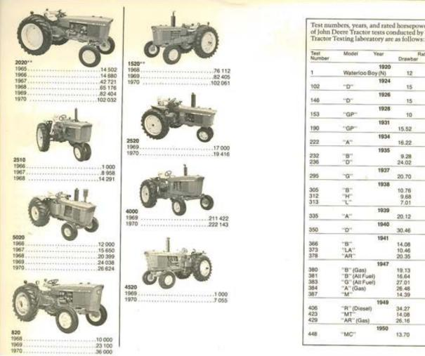
Test numbers, years, and rated horsepower results of John Deere Tractor tests conducted by the Nebraska
